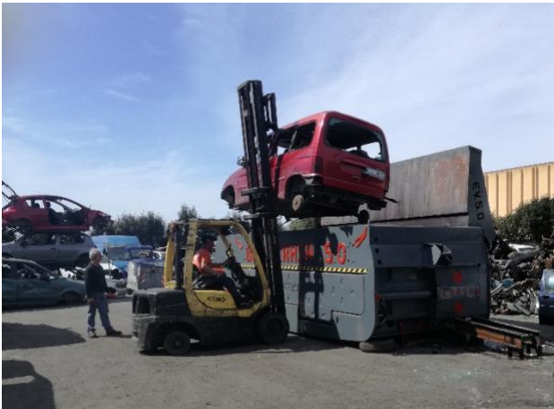
Possibility of loading with forklift
