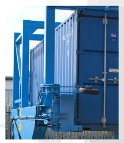
The container tilter is built around a fully welded steel chassis primarily from  $305 \times 305 \times 137$  kg beams.
