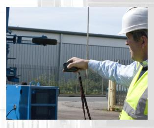
The unit comes complete with a radio controlled pendant remote unit, so the unit can be operated from the most advantageous and safe position. Manual override controls are also located on the machine as a backup system.
